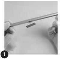
Fix optional steel plates (if using) with suitable countersunk screws (min. 4 steel plates per metre/40").
